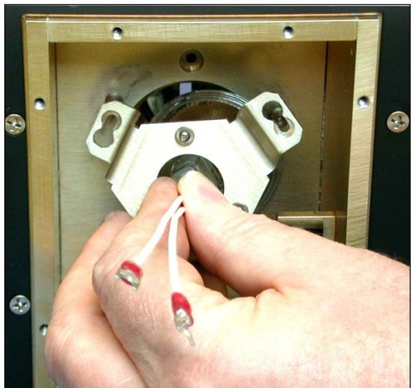
10. Place the lamp retaining ring over the shoulder screws, and rotate counter-clockwise (top side to left, bottom to right) to lock the lamp retaining ring into place.
