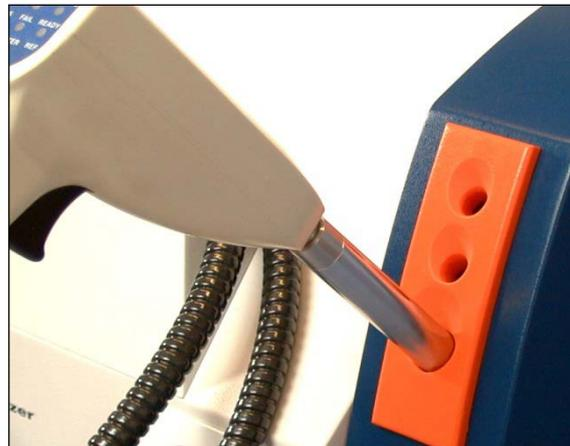
Reference Standardization is not technically required for the Interactance Immersion tip, because air is used as a reference, and it is assumed to be 100% transmissive.
