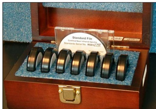
NIRStandards are designed for easy use with all Metrohm reflectance instruments used in the pharmaceutical industry, and most Metrohm instruments used in other industries. They are calibrated on our Master Instrument for use with the Instrument Performance Certification Program.
