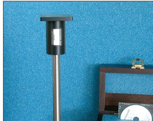
Vision prompts the user to rotate the Certified 99% Reflectance Reference. This is done to minimize the directional effects of the standard, and provide best consistency.
