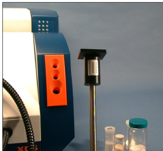
When instructed to scan the Wavelength Standard, or the Calibrated Reference Standard, simply press the door, and the holder will open.
