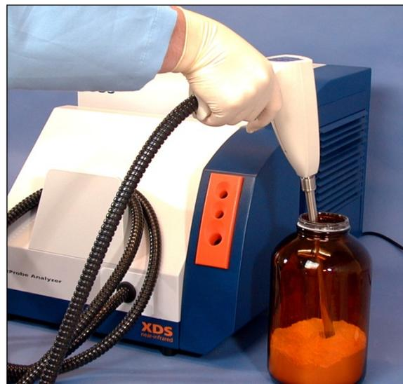
The probe barrel can be rinsed in a cleaning solution, then rinsed with distilled (or de-ionized) water to prevent sample carry-over from one barrel to the next.
