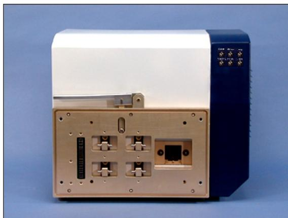
3. Open the right-hand panel of the instrument. Pull it gently by a fin, until the catch releases. This panel opens to about a 45-degree angle for access to connectors, and for filter inspection. Avoid scratches or damage.
