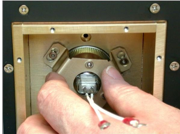
11. When the lamp is properly locked, the assembly will appear as shown. Note the shoulder screws holding the lamp retaining ring.
