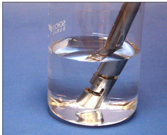
When finished sampling, the probe should be stored in the reference position. The probe end is protected from ambient light in this position. The end should be clean and dry when placed into the holder, to avoid drips and puddling inside the assembly. A small drain hole is provided, primarily to protect the instrument from accumulated drips.
