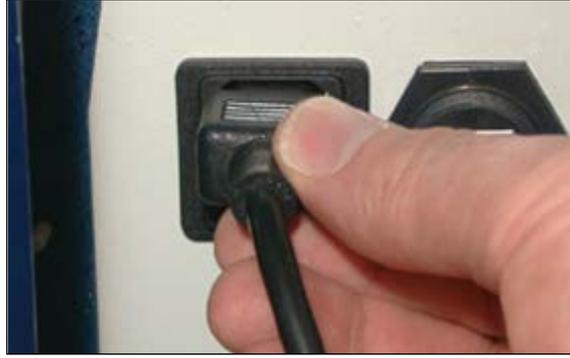
6. Attach the RJ-45 cable to the network connector on the instrument. If using Direct Connection, use the gray cable from the instrument accessory kit.
