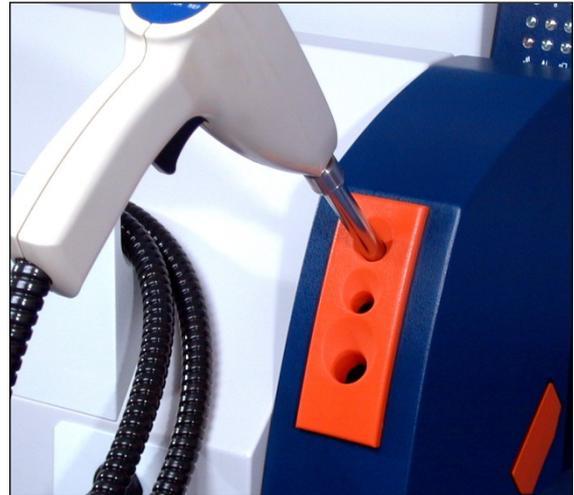
With the Interactance Reflectance probe barrel mounted, the operator may sample powders in shipping containers, barrels and drums.
