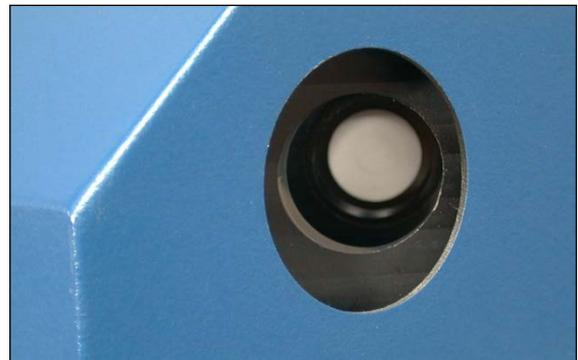
9. Reach in with a tissue, then press the reflectance standard out from the other side -- insert the Smart Probe gently into the reference position. The standard should pop out into the tissue.
