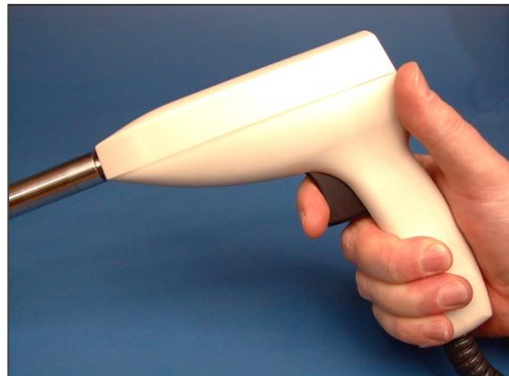
The fiber optic bundle, while well-protected, should always be handled with care. The individual fibers are quite thin, and can be broken by rough handling. Breakage of these strands will reduce the light energy, and will eventually cause the instrument to fail diagnostic tests.
