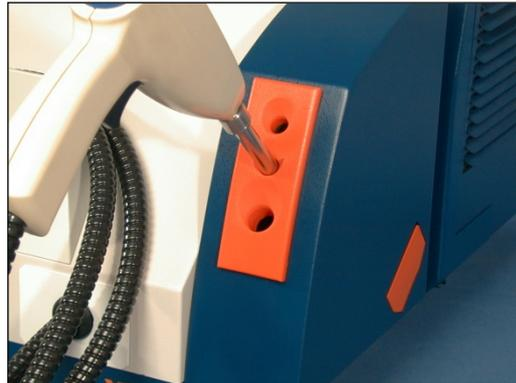
Close the drawer first, then gently lower the Smart Probe, into light contact with the standard window.
