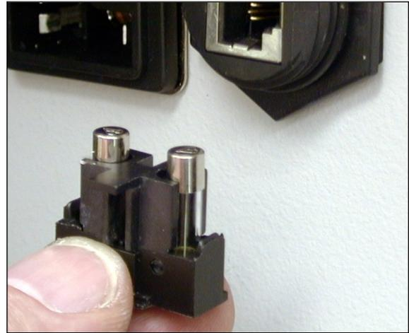
Close the fuse door fully. Plug the AC power cord in. (Plug the RJ-45 cable in if it was removed.)
