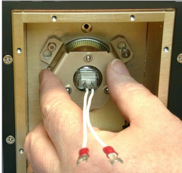
5. This photo shows the lamp retaining ring in the removal position. The spring will tend to push the retaining ring outwards when the shoulder screws line up with the openings. Do not drop the lamp or retaining ring.
