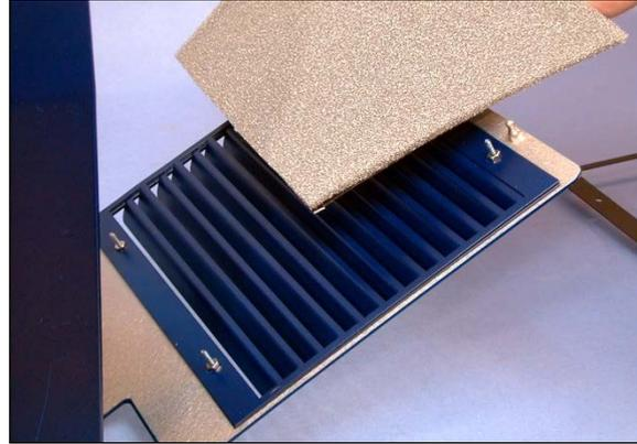
Install the new, clean filter material carefully over the screws as shown. The screws should penetrate the filter material fully.
