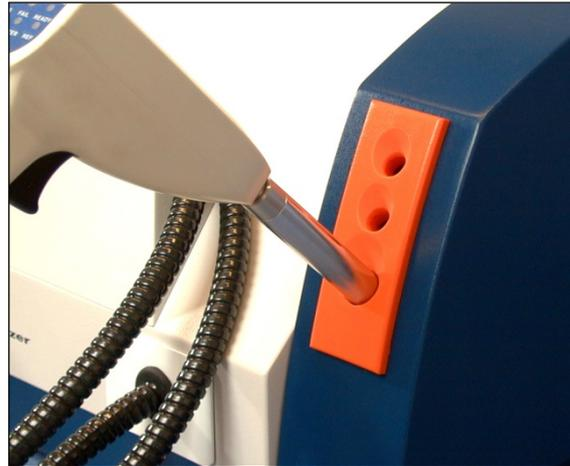
When placing the Interactance Immersion (Liquid) Tip into the sample, angle it slightly to avoid trapped bubbles between the mirror end and the sample window. Bubbles will change the spectral readings.
