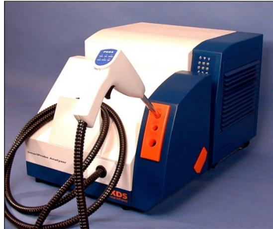
Instrument Calibration makes use of an external wavelength reference. The reference mounts in a cup holder on the side of the instrument as shown. (Leave room for easy access.)
