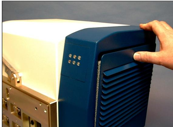
8. Position the sampling module directly in front of the monochromator.
