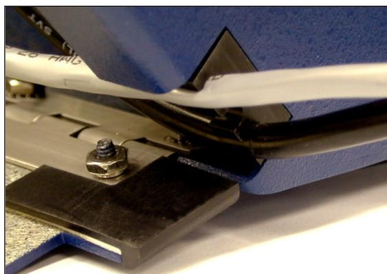
5. Insert the AC power cable into the AC power block as shown.
