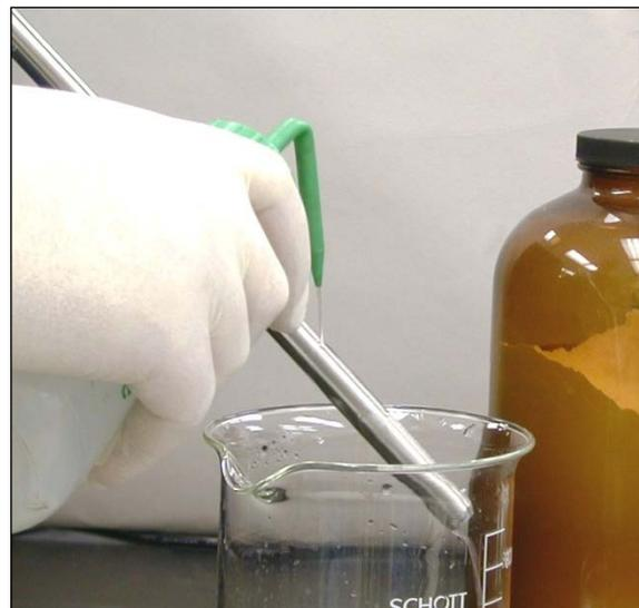
When finished sampling, the probe should be stored in the reference position. This is the proper position for Performance Test, Gain Test, and Wavelength Linearization.
