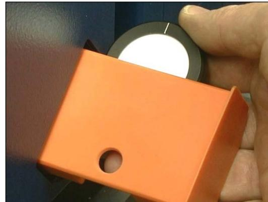
When the test is complete, a spectrum of the standard is shown in the upper right quadrant of the screen. A tabular report is shown in the lower right quadrant, giving each peak, its nominal position and its measured position. The difference from nominal, and the repeatability of wavelength peak positions are calculated.
