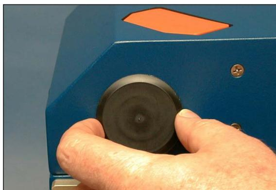
5. Lift the sample drawer upward, out of the way. (Hold in this position.)
