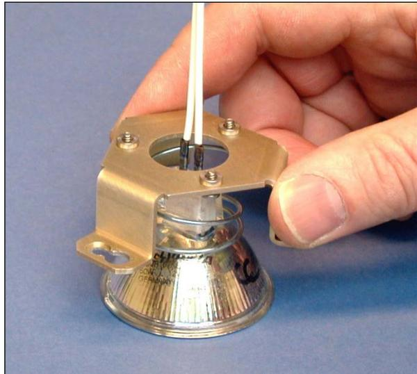
9. Gently place the lamp and retaining ring into the lamp box in the instrument.
