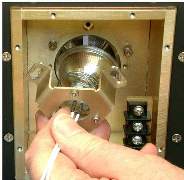
7. With the lamp wires straight, lift the lamp retaining ring upward and off the lamp as shown.
