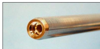
Do not scratch the Smart Probe window. Scratches will cause scattering of signal, and may affect analytical results.
