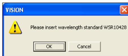
Insert the WSR10xxx Wavelength Standard Cell when prompted. Insert the cell in a consistent rotational position for repeatability.
