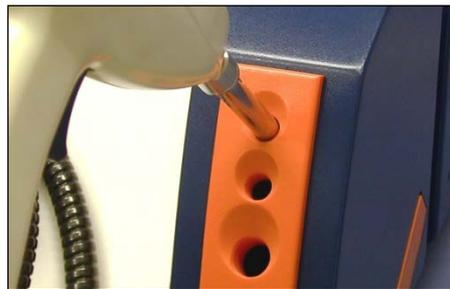
When prompted, squeeze the trigger on the Smart Probe handle to start Performance Test.
