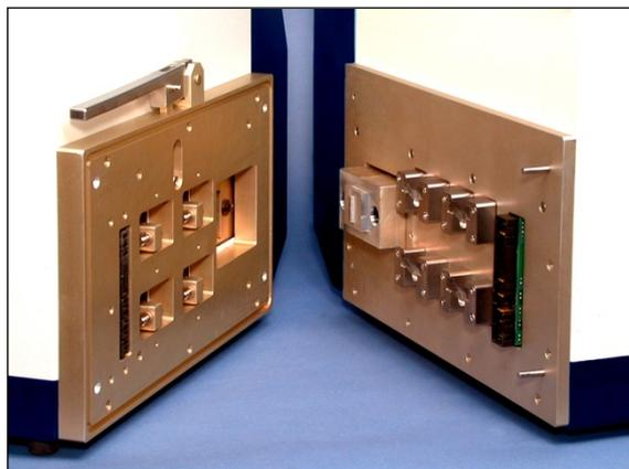
9. Lift the release handle on the monochromator and engage the module “catches” to the locking togs on the monochromator. (Module not shown to allow a good view of handle.)
