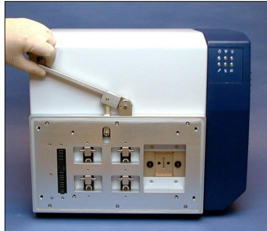
2. When lifting the monochromator, place arms on either side of unit as shown.
